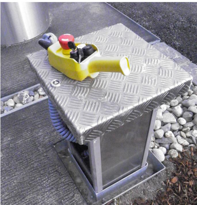
Retractable control column with control bulb
