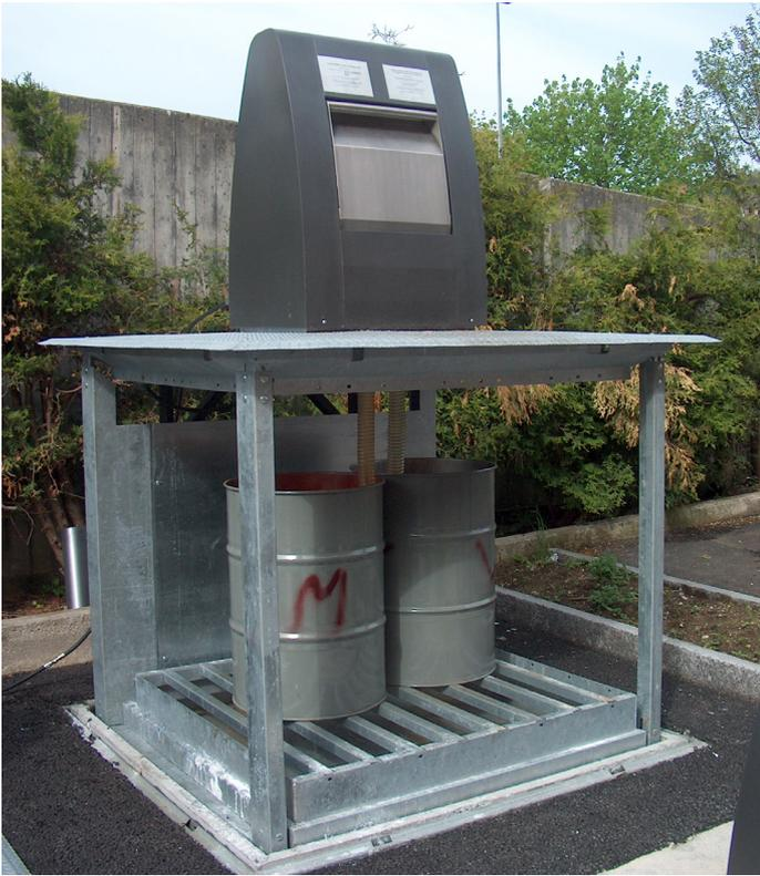
Collection Point for used oil with two barrels à 159 l
