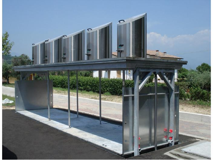
The existing infrastructure is gently lowered from the surface into the underground. Conventional collection containers are placed on a hydraulically driven auto hoist and can be emptied with a conventional emptying vehicle.
